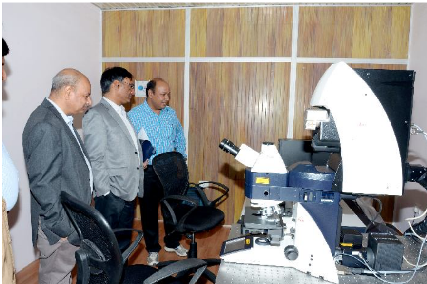
Nesly installed Raman Spectrometer System (Model-RENISHAW InVia Reflex) useful for determining the chemical composition and structure of sample, whether, solid, liquid, gas, gel, slurry or powder
